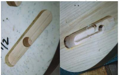
The electronics rout is 1 1/2 inches deep. And The jack hole on
