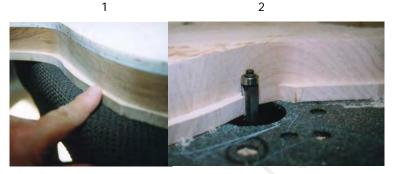
Once the entire circumference of the body is routed you can remove the template. Set-up the router with the second straight cut bit, the one with the bearing on the bottom. Extend the bit so that the bearing will track along the previously routed edge of the body. See #2 above.
