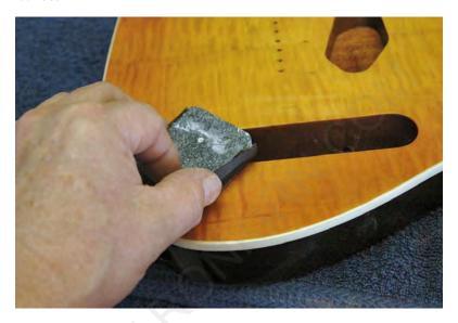
Once the surface looks uniformly flat, dry the surface thoroughly and check by looking at the surface with something bright reflecting off it.
